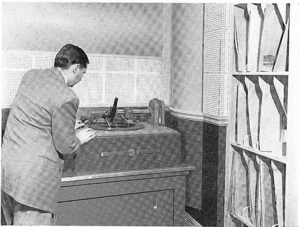
FIG. 3. Photos at left show two views into the combined recording room and studio A control room. Control equipment consists of an RCA Type 76-C Console and Type BCS-1A Studio Switching unit. Lower photo shows the Type 73-B Professional Recorder in use.
