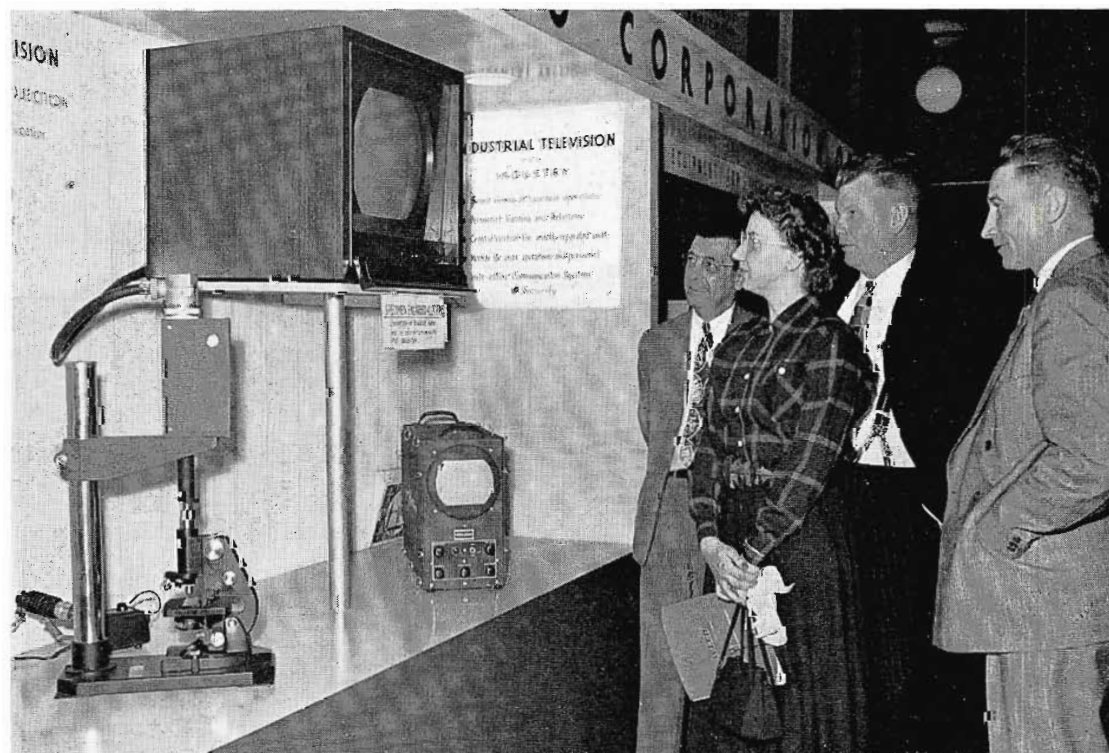
VIDECON EQUIPMENT is complete in these two units. The camera proper is only a little larger than a 16mm movie camera. The control unit which contains the sync generator, deflecting circuits, video amplifiers, controls and monitor kinescope is the same size as one of RCA's standard field units.
