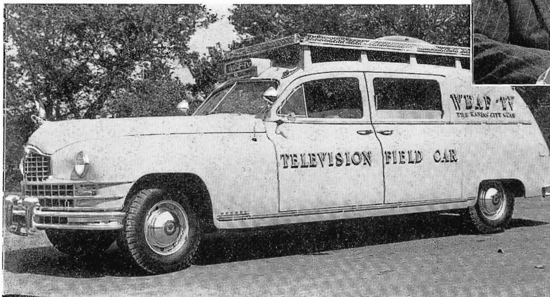
FIG. 11. Below is WDAF-TV custom built field car which carries the field pickup gear. Microwave relay dish is transported on roof of car.
